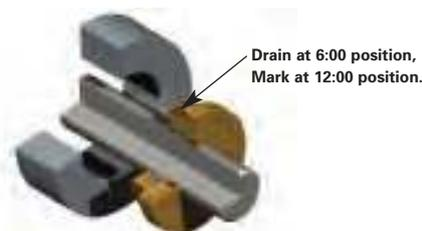
**Figure 15: Drain Port Positioning**
